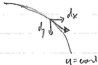
$$\begin{aligned} du &= \frac{\partial u}{\partial x} dx + \frac{\partial u}{\partial y} dy \\ &= (dx, dy) \begin{pmatrix} \frac{\partial u}{\partial x} \\ \frac{\partial u}{\partial y} \end{pmatrix} \end{aligned}$$
